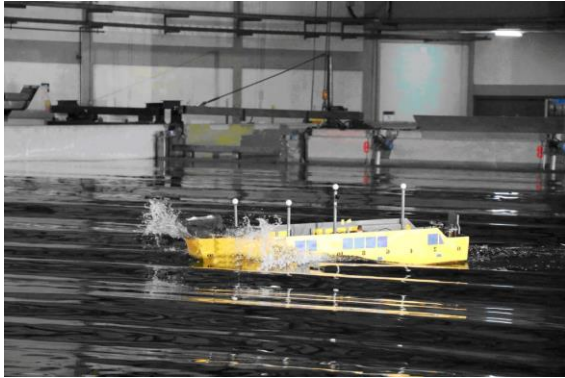
Gambar 7. Proses pengujian seakeeping Model Kapal Ferry Ro-Ro 750 GT heading 135 deg
