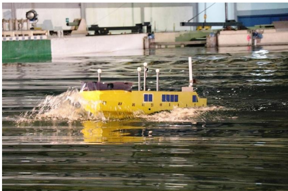
Gambar 8. Proses pengujian seakeeping Model Kapal Ferry Ro-Ro 750 GT heading 180 deg
