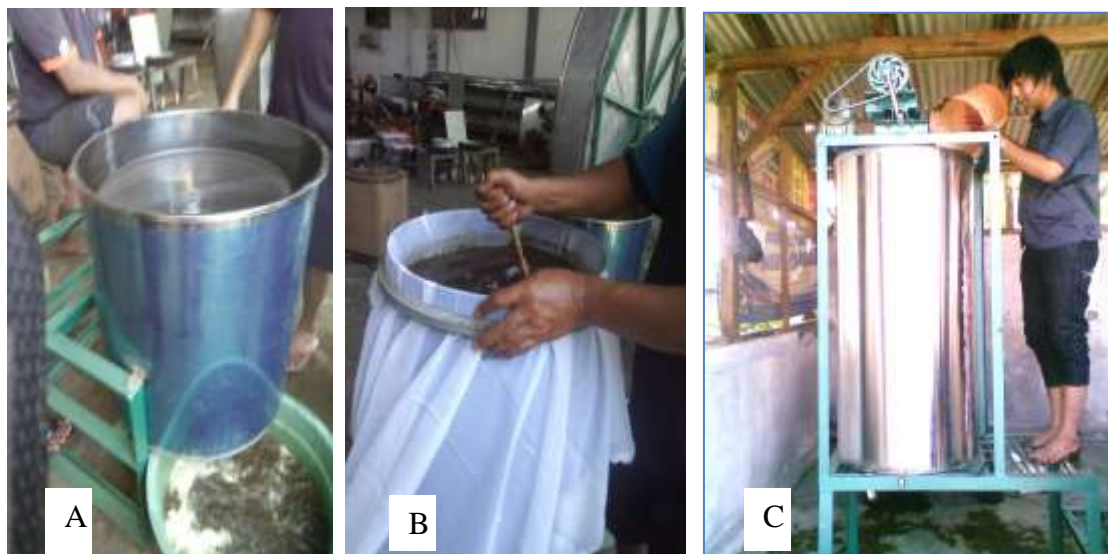
Figure 2. The mature compost was extracted with water then A. The mixture of composts was extracted with water then was centrifuged at 1000-2000 rpm to separate the coarse compost with the smooth particles, and B. Filtrate was strained with fine strain cloth to produce very fine particles of compost, so it will not clog the nozzle sprayer (Wahyuni et al. 2016b). C. The strained water compost was put into the mixer tank after added with Pseudomonas putida H10. The mixer was rotated for 30-60 minutes / day, for one week then ready to use as biopesticide (Wahyuni et al. 2013).
