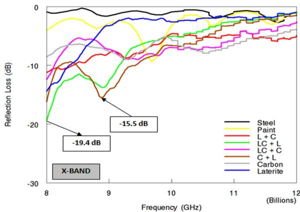
Fig. 6. Microwave reflection losses of the samples at 8-12 GHz
