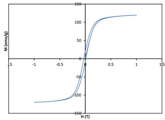
Fig. 4. Hysteresis loop at room temperature of pure laterite
