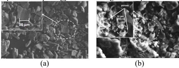
Fig. 2. SEM images (a) laterite and (b) active carbon
