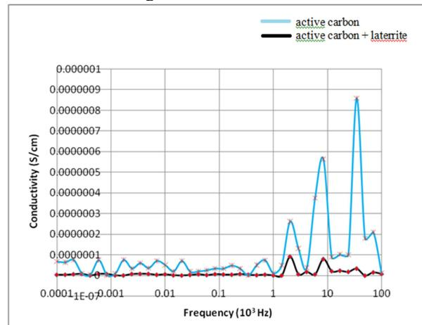
Fig. 5. Conductivity of active carbon as a function of frequency
