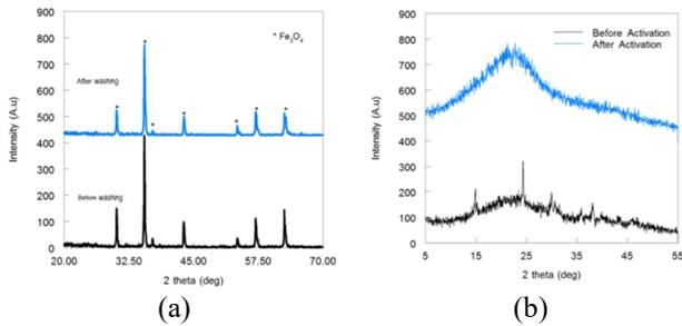
Fig. 1. XRD pattern of the (a) Laterite and (b) Activated Carbon
