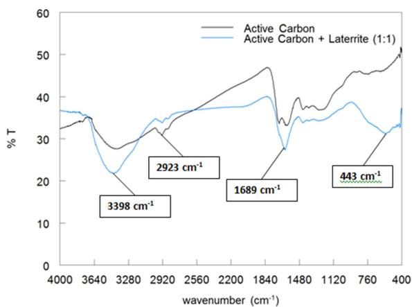
Fig. 3. FTIR spectra of active carbon and active carbon + laterite (1:1)
