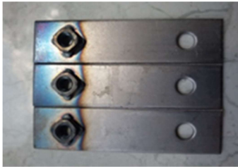
Figure 2. SPCCSD 1.8 plate and Nut weld M6 after welding
