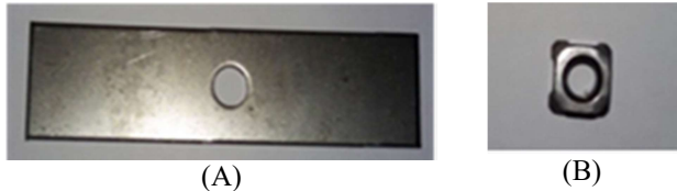
Figure 1. A. SPCCSD 1.8 plate B. Nut weld M6
