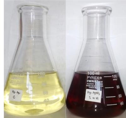
Fig 1. The Change of solutions during tge bioreduction of AgNO 3 into AgNPs using Hydrodictyone sp. extract a. control b. the solution after 18 hours
