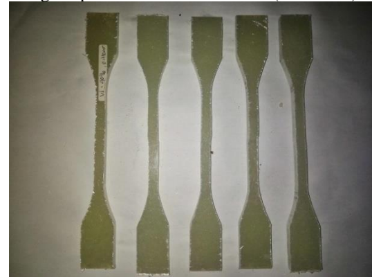
Gambar 1. Spesimen uji tarik standar ASTM D 638-02a
