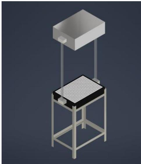
Gambar 2. Desain Mesin *Vacuum forming*
