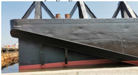
Gambar 4. Vertical side finish coating
