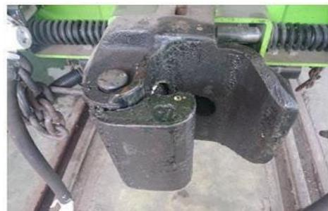
Gambar 2. Tightlock Automatic Coupler [7]
