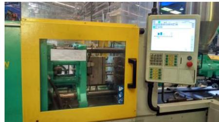
Gambar 2. Mesin *Injection Molding* ARBURG All Rounder
