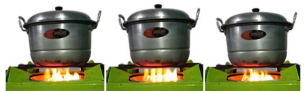
Figure 5. Flame characteristics without adjuster
