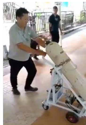
Figure 8. Testing the performance of the electric trolley on a road slope of 5°
