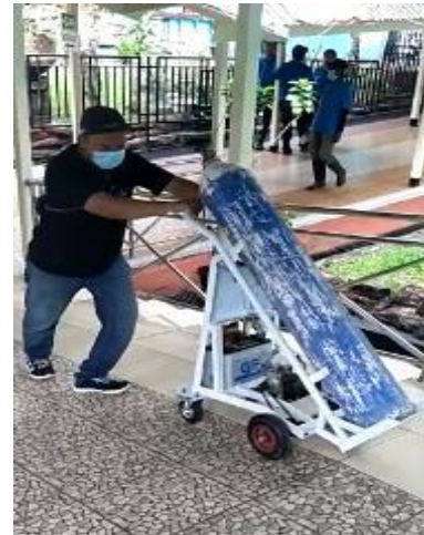
Figure 11. Testing the performance of the electric trolley on a road slope of 10°
