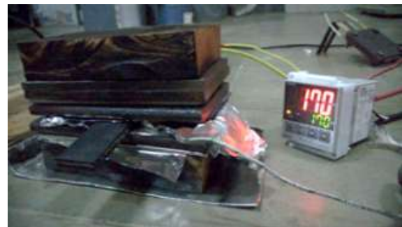
Gambar 3. Proses pemanasan belt
