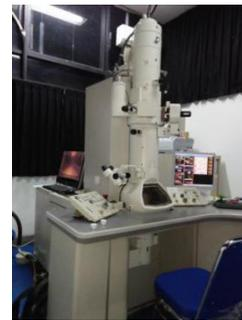
Gambar 4. Alat TEM merk Jeol type JEM 1400.
