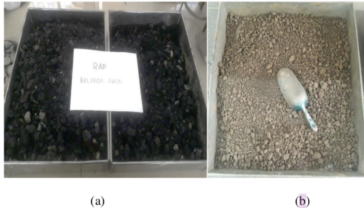
Gambar 2 Material Penelitian (a) Material Pasca Bencana Palu, (b) Asbuton Butir Lawele
