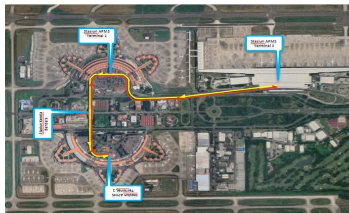
Gambar 1 Layout Jalur Perjalanan Kereta Automated People Mover System Bandar Udara Internasional Soekarno – Hatta
