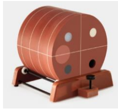
Gambar 3. Gammex ACR 464 phantom
