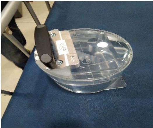
**Gambar 2.** Phantom bawaan *CT-Scan* GE
