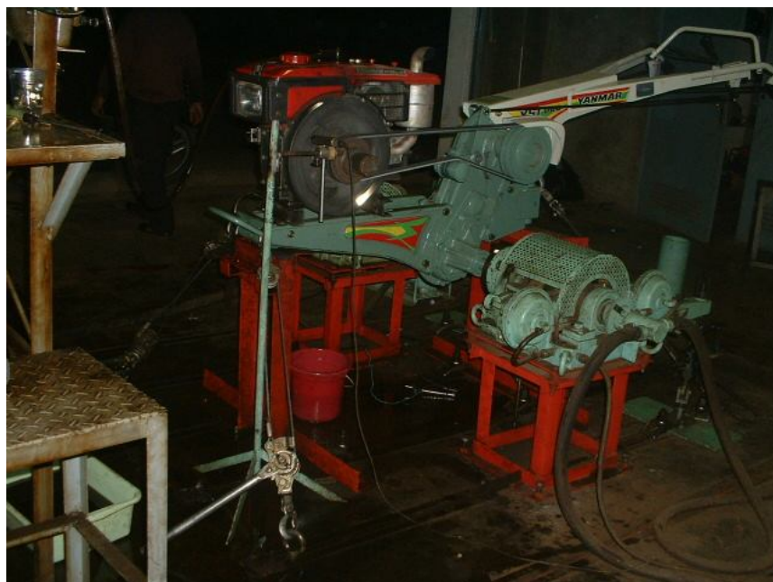
Gambar 9. Instalasi uji laboratorium mesin diesel berbahan bakar coco-biofuel
