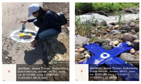
Figure 2. Marking and reading of GCP points
