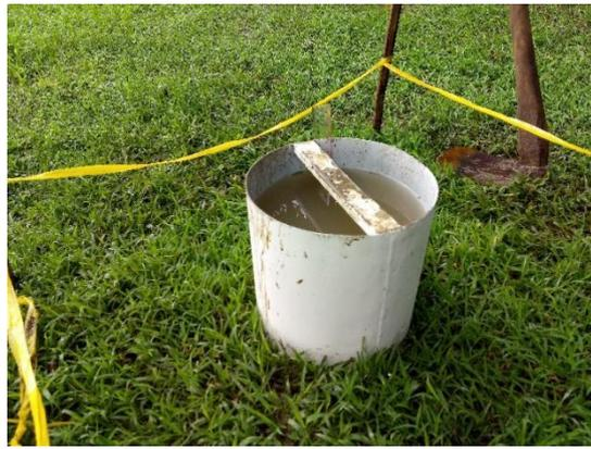
Figure 3. The soil infiltration measurement on the test plot
