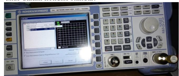
Gbr. 8 Proses kalibrasi network analyzer
