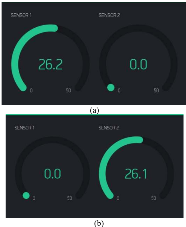
Figure 3. Water Gauge Display at Blynk a) Pipeline 1, b) Pipeline 2
