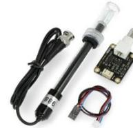
Gbr. 6 Sensor Salinitas *Electrical Conductivity*
