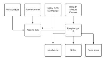
Fig 1 . ITS System Block Diagram
