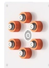
Gbr 7. Desain 3D Stator Motor BLDC 3 \phi Axial Flux Tampak Belakang
