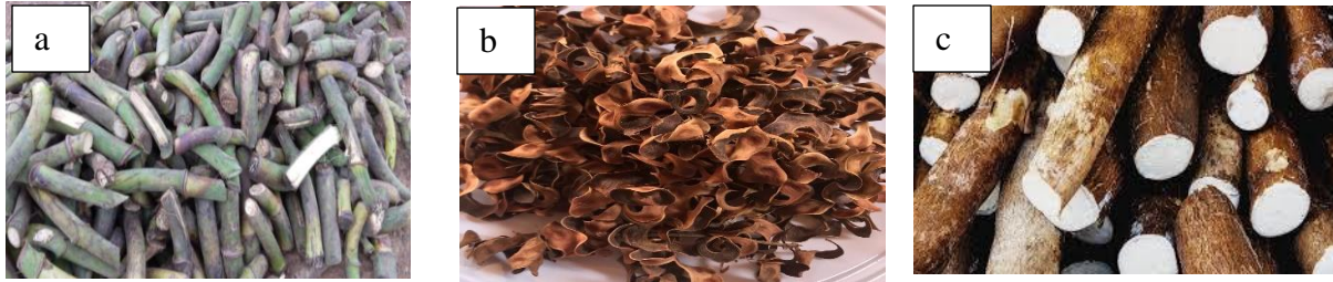
Figure 1. Biomass and binder raw materials (a = Plantain peduncles, b = Acacia mangium pods, c = cassava)
