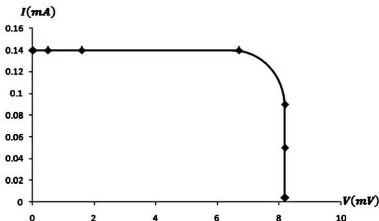
**Figure 7.** The graph of Cu-  $MoS_2/g - C_3N_4/Cu_2O$  photoelectrochemical solar cell after surface modification
