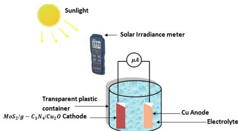
**Figure 2.** Illustration of the fabricated Cu –  $MoS_2/g - C_3N_4/Cu_2O$  Photoelectrochemical solar cell
