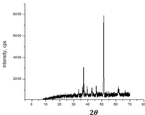
**Figure 3.** XRD pattern of  $MoS_2/g-C_3N_4/Cu_2O$
