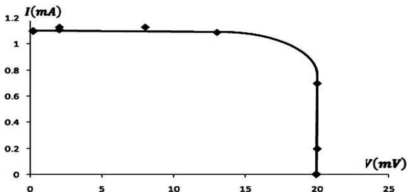
**Figure 6.** The graph of Cu- $Cu_2O$  photoelectrochemical solar cell before surface modification
