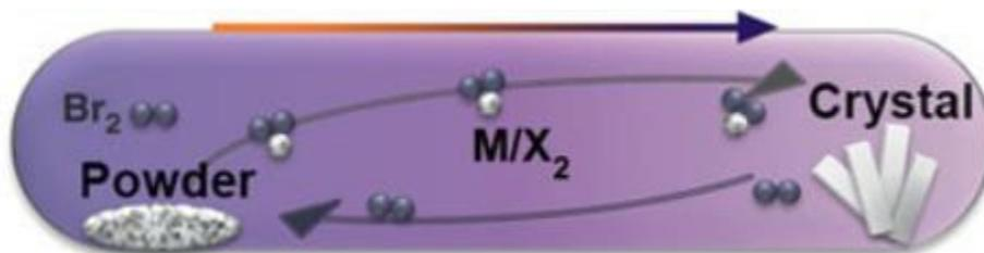
**Figure 3.** Chemical vapour transport [29]
