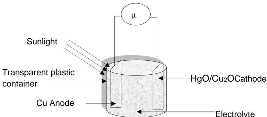
**Figure 4.** Diagram of the made-up HgO/Cu<sub>2</sub>O Photoelectrochemical solar cell
