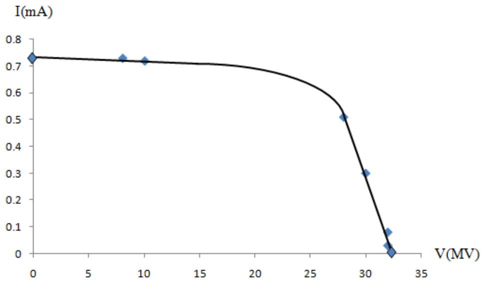
**Figure 6.** The graph of current-voltage features of synthesized  $\text{HgO}/\text{Cu}_2\text{O}/\text{HgO}$  after deposition of  $\text{HgO}$
