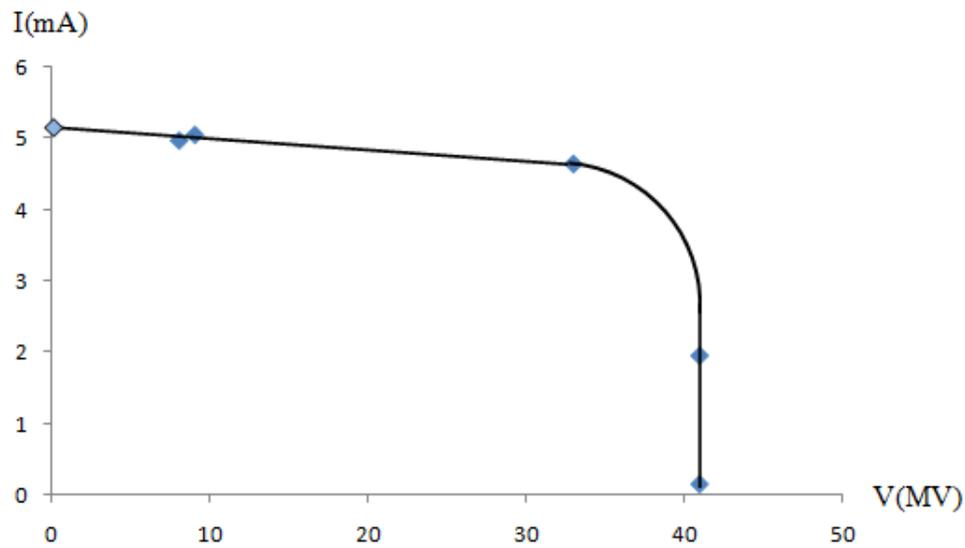
**Figure 5.** The current-voltage features of synthesized  $\text{Cu}_2\text{O}$  before deposition  $\text{HgO}$
