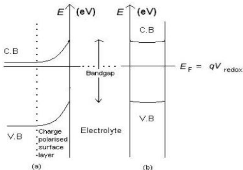
**Figure 1.** Graphical representation arrangement of a charge-polarized facade layer in PECs photovoltaic cell[29]
