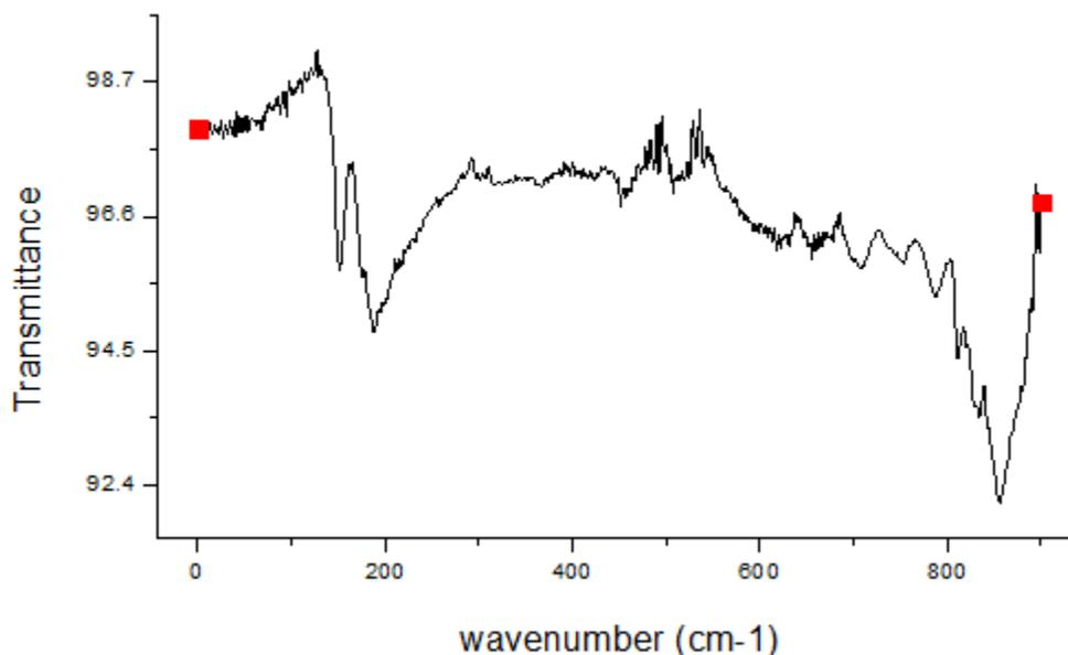
**Figure 7.** The FTIR of Deposited Mercury oxide in a furnace on pinnacle of  $\text{Cu}_2\text{O}$  substrate
