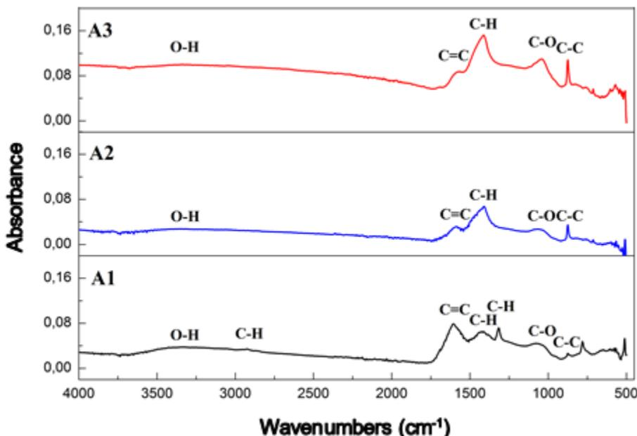
**Figure 2.** FTIR spectra of carbon derived from water hyacinth at carbonization temperature 400°C (sample A1), 500°C (sample A2), and 600°C (sample A3)
