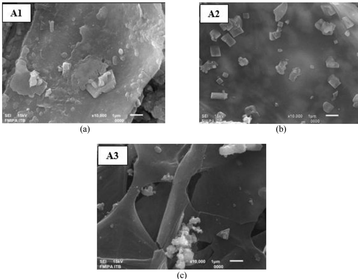
**Figure 1.** The surface morphology of carbon derived from water hyacinth at carbonization temperature (a) 400°C (sample A1), (b) 500°C (sample A2), and (c) 600°C (sample A3), respectively
