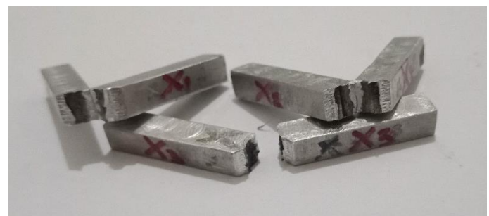
Gambar 6. Hasil uji Impak kelembaban 84%
