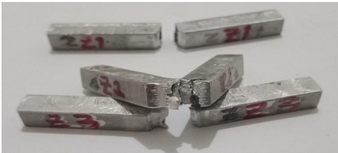
Gambar 8. Hasil uji Impak kelembaban 77%
