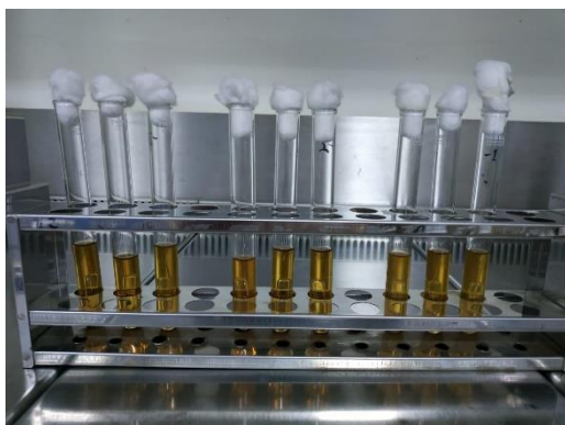
Figure 1. Coliform Estimation Test for SNI ISO 9308-1:2014; The results were negative, indicated by no color change and no gas in the Durham tube.
