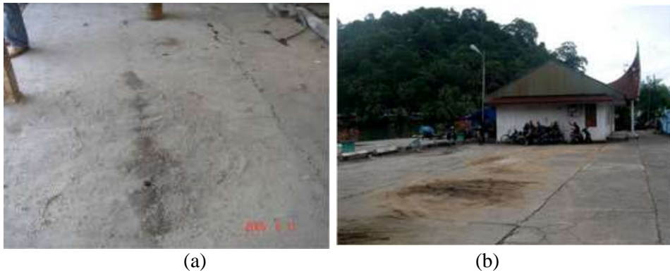
Figure 1. (a). Silty sand liquefaction at UMY campus during the 2006 Yogyakarta earthquake. (b). Silty sand liquefaction at Padang airport during the 2009 West Sumatera earthquake
