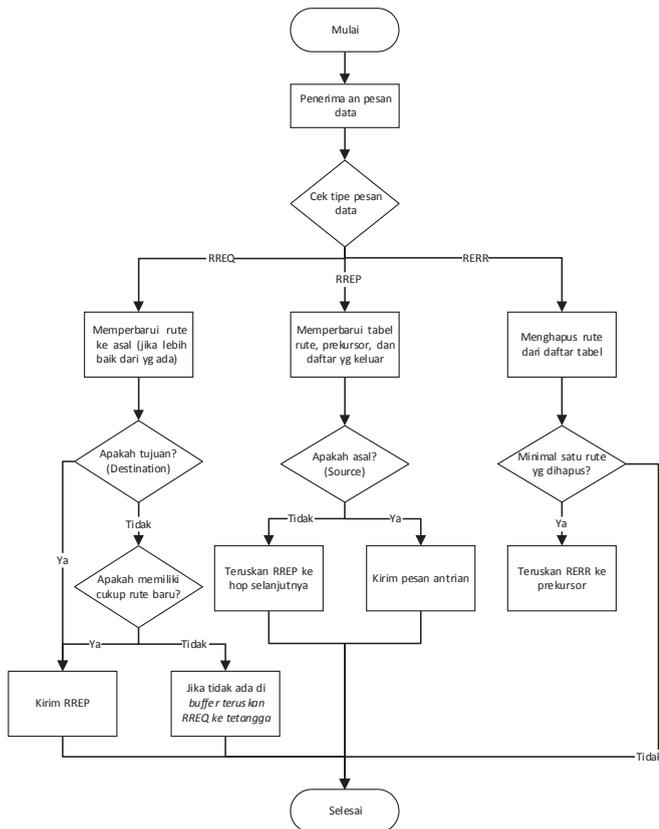
Gbr 4. Diagram alir mekanisme routing AODV
